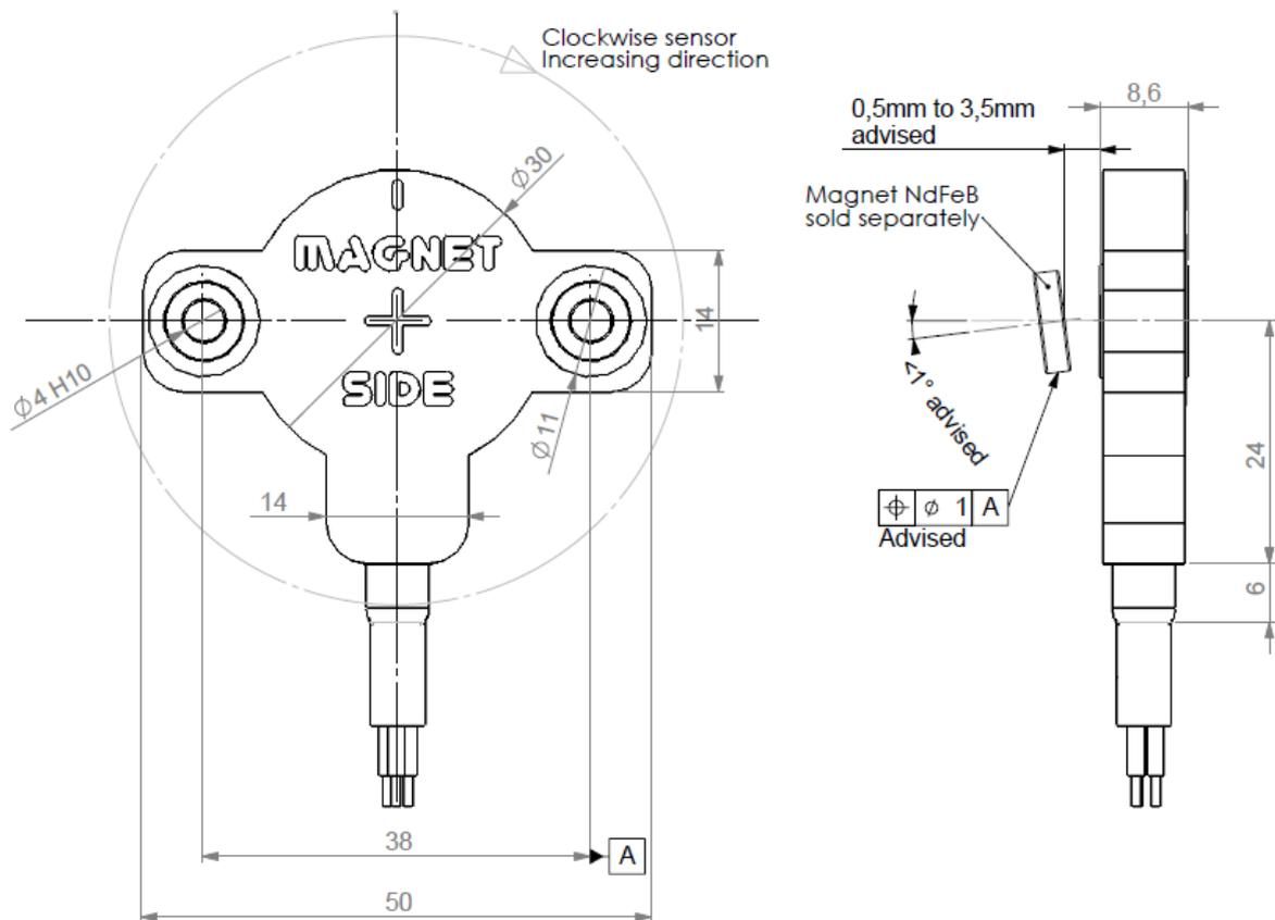
Shaft system with magnet to be ordered separately (cf specific data-sheet).
