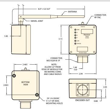
The SwiftComm Receiver Module has an MS connector that provides the same output signals as a standard BEI encoder. Input power can be from 5 to 28 VDC. Quadrature output signals (specified at time of ordering)
